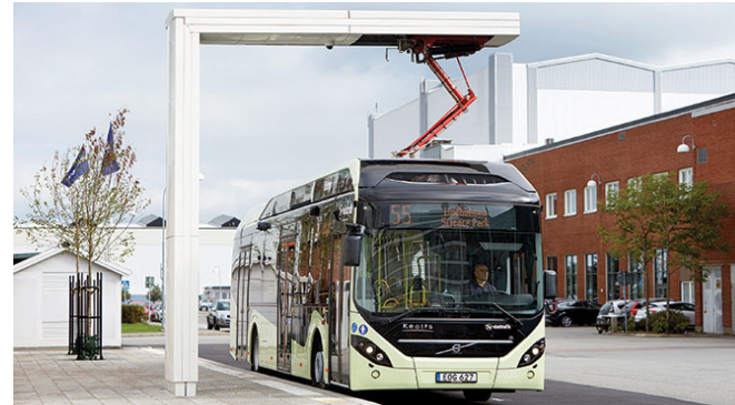
Figure 6.22: Electric Vehicle Charging Station for Buses
