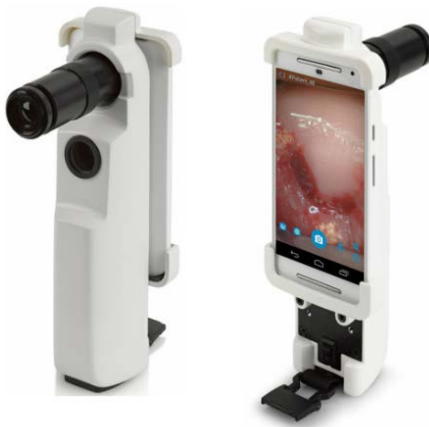
Figure 4-5-2. MobileODT EVA System
