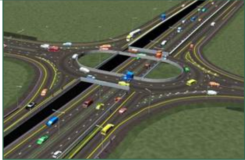
Geri-Alimi Split Diamond Underpass
