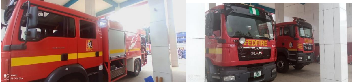
Pictures 55: Procured Water/Foam Fire-Fighting Equipment of 5000/1000 litres Foam Tank
