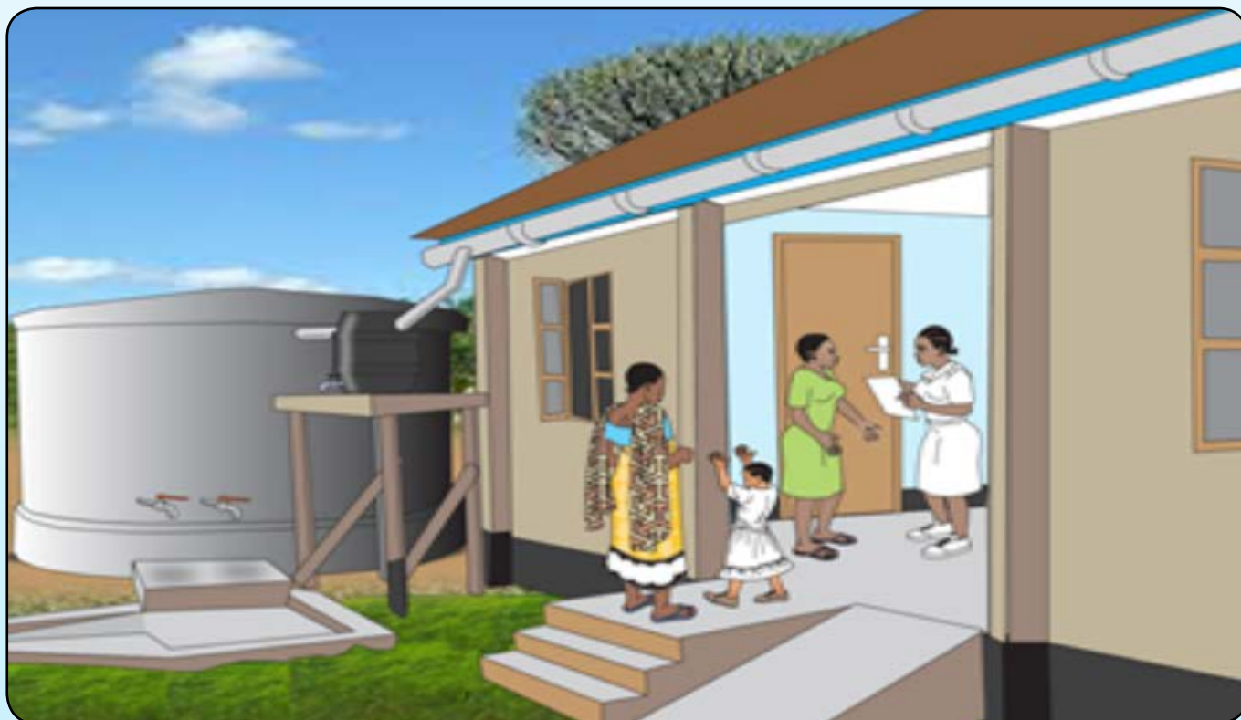
Figure 5.4: Rain water harvesting with first -flush tank
