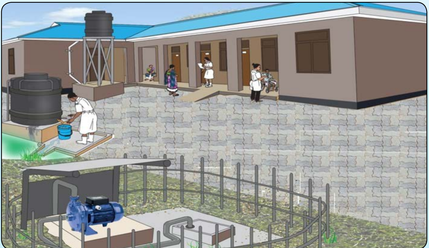
Figure 5.5: Water abstraction point at a dispensary
