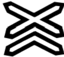
LEVEL CROSSING WARNING CROSS-TWO TRACKS
