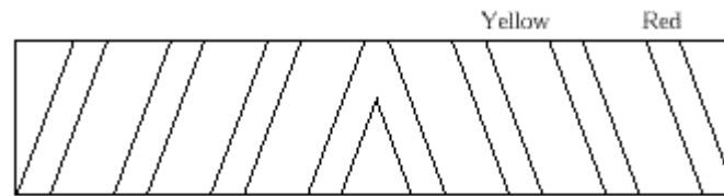
Form of Warning Sign--(Chevron Pattern)
