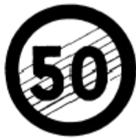
De-restriction sign indicating end of the speed limit shown and as imposed by a previous regulatory sign.
