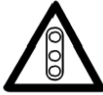
TRAFFIC SIGNALS AHEAD Signals (in descending order) Red, amber, green reflectorized
