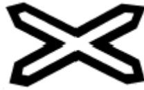
LEVEL CROSSING WARNING CROSS-ONE TRACK
