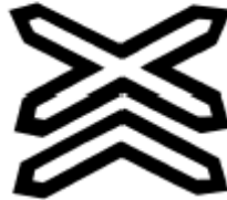
LEVEL CROSSING WARNING CROSS-TWO TRACKS
